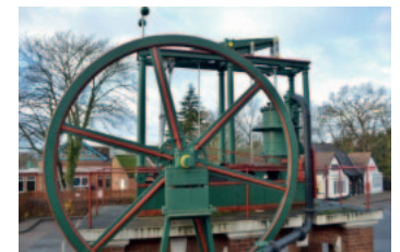
A preserved Watt beam engine at Loughborough University.
